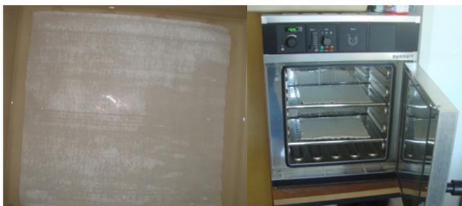
Figure 2. a) knitwear sample in water bath, b) knitwear sample in drying machine FAST 4
